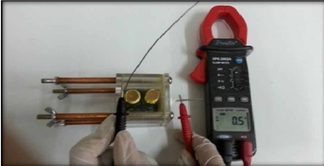
Form [5] measuring voltages when eight days of an MFC application system period
